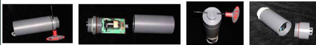
Figure 4, Removing logger case (left: original model, right: new design)
